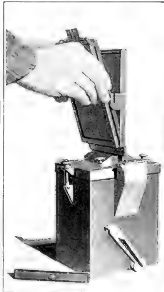
Placing the camera plate-holder in the transferring-hopper for its entrance into the tank. It is securely held in place by a lock-bar. Afterwards the plates are washed and placed in the fixing bath in the same way for fifteen minutes
